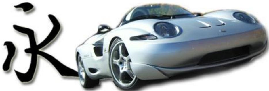
The Triposto is built on a Porsche 911 chassis, with a 1988 Porsche six-cylinder engine and a gearbox from the latest generation 915 series. Kwok and his team concentrated on design and aerodynamics, the engineering professor's specialty. Much of the chassis is rebuilt, however, and the sci-fi "skin" of the vehicle is painstakingly designed for maximum aerodynamic efficiency, but also for style, by some of Quebec's top young automotive and industrial designers recruited by Kwok.
